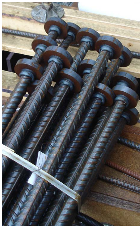
HRC 150 used for reinforcement of shear keys
